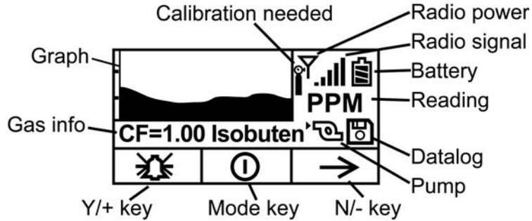
During sampling, the display's readings are shown numerically, plus the graph tracks the highest readings over time. The numeric reading alternates between the value and the measurement units, as well:
