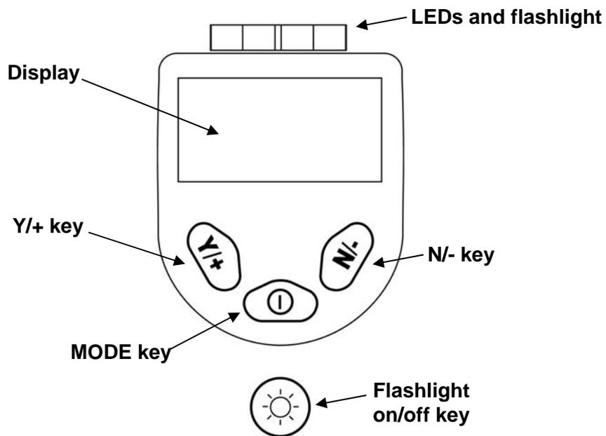
In addition to their labeled functions, the keys labeled Y/+, MODE, and N/- act as “soft keys” that control different parameters and make different selections within the instrument's menus. From menu to menu, each key controls a different parameter or makes a different selection.
